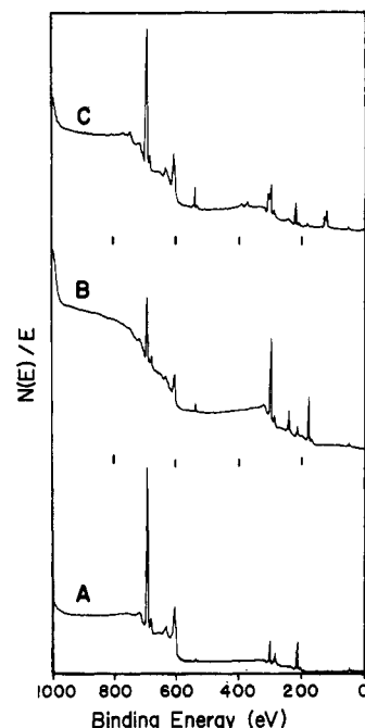
Figure 6. XPS survey spectra for the synthesis of PCTFE-CHO. The reaction of PCTFE with 2-lithio-1,3-dithiane was carried out in 50:50 heptane/THF at -78^{\circ}\text{C} for 60 min. The takeoff angle was 75^{\circ} from the film surface. A. PCTFE; B. PCTFE-DT; C. PCTFE-CHO.
